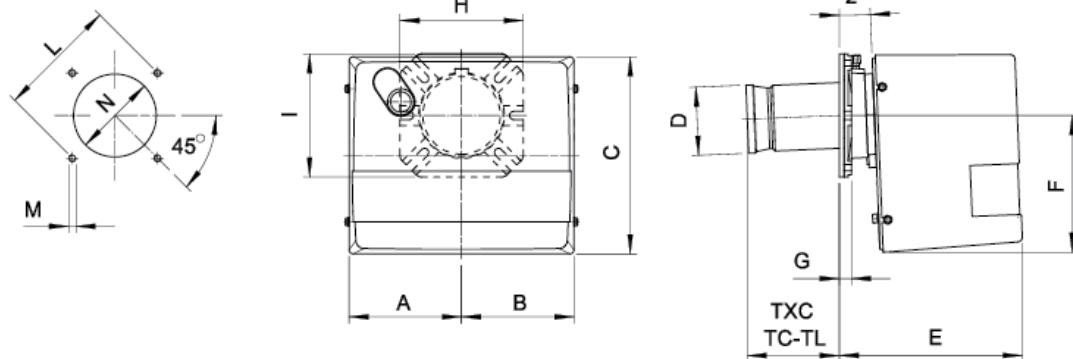
\* Suggested dimension of connection between burner and generator
