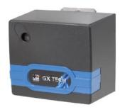
Light oil burners at 2 stages at 2 steps pressure – Low NOx (NOx < 120 mg/kWh). Frame made in aluminium, sound-attenuated protection cover, high efficiency combustion head with micrometric adjustment, high flame stability and low emissions.
