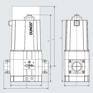
e = space required for replacing the solenoid
