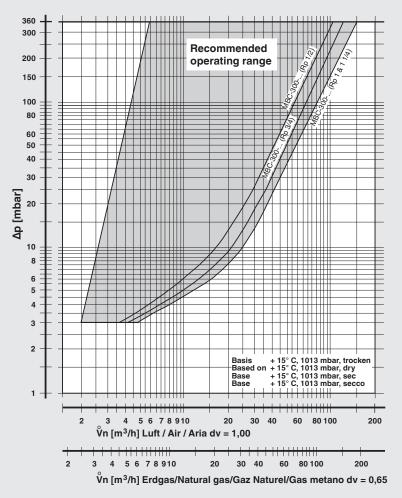
Volume flow pressure difference characteristics in steady state with microfilter.
